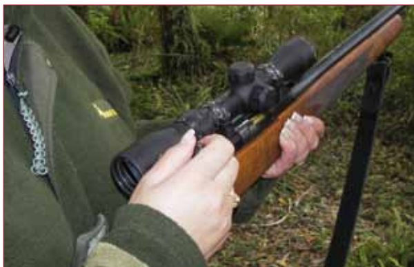
Figure 2: The cartridge must be removed if the game gets away without the shot being fired.
